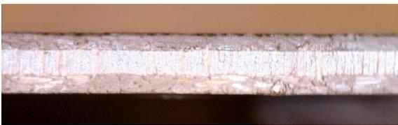
Post Laser Singulation where the process has been controlled appropriately. The quality of the cut is obvious and the degree of expansion and charring of the top layer is zero. Cut speed for this operation was >35mm/second with a single pass. This results in an effective cutting speed of >35mm/sec.
