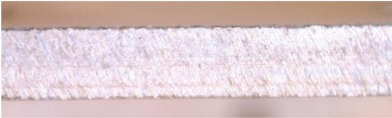
Edge of panel from manufacturer. This shows a clean aluminum substrate, a thin synthetic material layer on top. This is prior to assembly or singulation operations.
